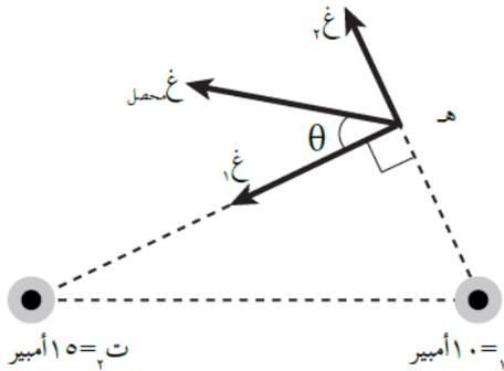
$$G_1 = \frac{\mu_0 I_1}{\pi r_1} = \frac{10 \times 10^{-7} \times \pi \times 4}{0,3 \times \pi \times 2} = \frac{2}{3} \times 10^{-4} \text{ تسلا}$$
