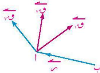
$$\begin{aligned}\vec{r} &= \vec{B} - \vec{A} = (1, 2) - (0, 0) \\ \vec{c} &= \vec{r} \times \vec{F}_1 \\ &= (2, 1) \times (1, 2) \\ &= (1+4) \vec{i} - (1+4) \vec{j} \\ &= 5\vec{i} - 5\vec{j} \\ \vec{F}_2 &= \vec{r} \times \vec{F}_2 = (1, 2) \times (1, 6) = (1+6)\vec{i} - (1+6)\vec{j} \\ &= 7\vec{i} - 7\vec{j} \\ \vec{F}_3 &= \vec{r} \times \vec{F}_3 = (1, 2) \times (4, 4) = (4+8)\vec{i} - (4+8)\vec{j} \\ &= 12\vec{i} - 12\vec{j}\end{aligned}$$
